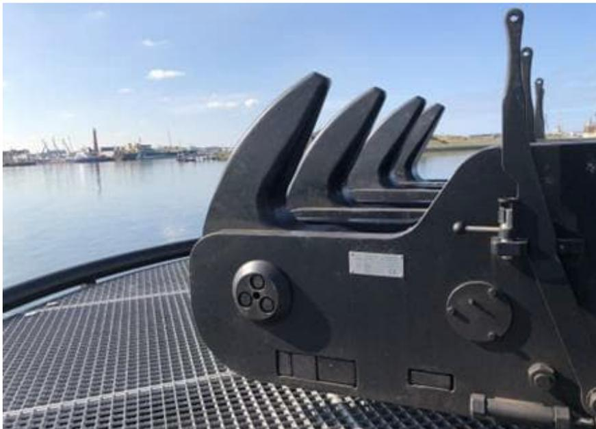
Figure 6-1 Example Quick Release Hook (Source: Straatman)
