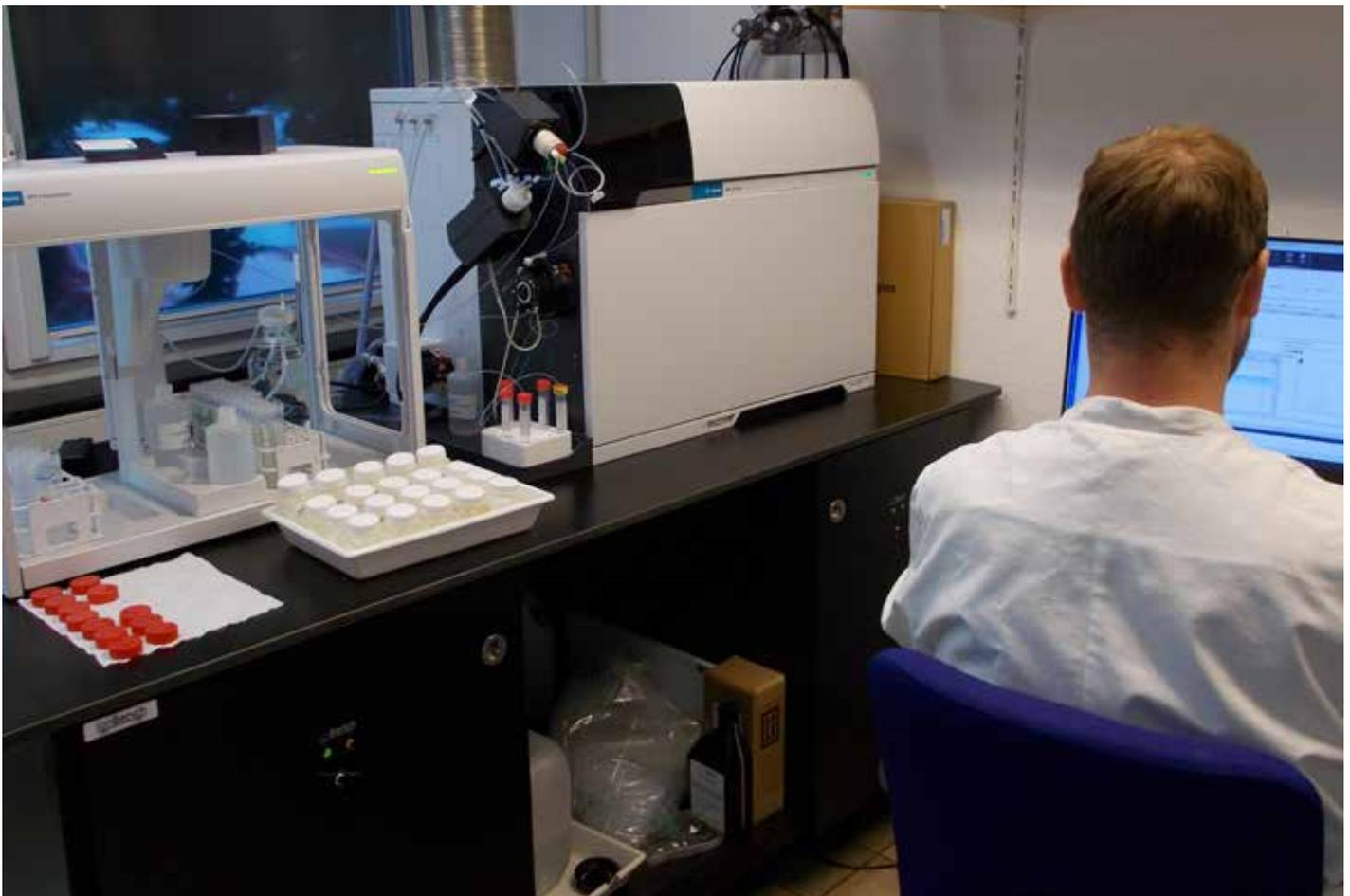
Abb. 2: Moderne Metallanalyse mittels ICP-MS (Inductively Coupled Plasma Mass Spectrometry) (NLWKN)
